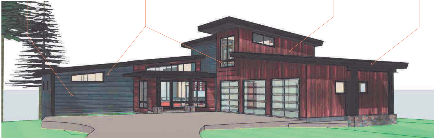
BRIDGER STEEL BOX RIB 7.2 STRUCTURAL SIDING COLOR DARK GRAY OR SIM.
